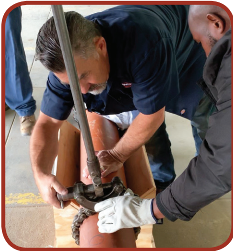
Figure 17: Use of a chain snap cutter is demonstrated in a VCP operations and maintenance workshop.
