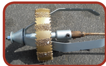
Figure 14: An example of a root-cutting device used with a mechanical rodder.
