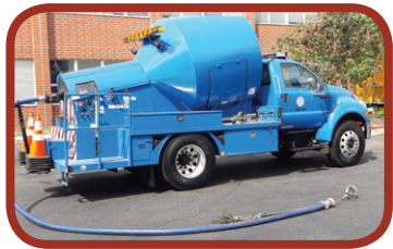
Figure 13: A mechanical rodding machine has 1,200 feet of continuous rod. Photo provided by Haaker Equipment Company.
