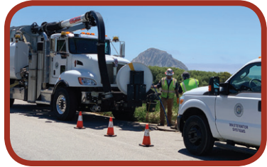
Figure 15: A Morro Bay, CA combination sewer cleaning truck being used to hydro-flush and vacuum sewer lines.
