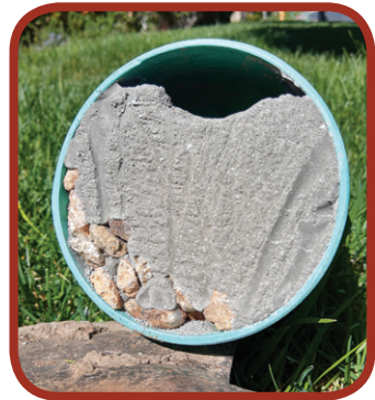
Figure 3: Construction concrete is found in many locations.
