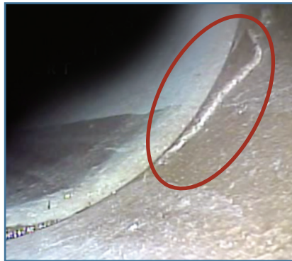
Figure 28: Surface imperfection created during extrusion
