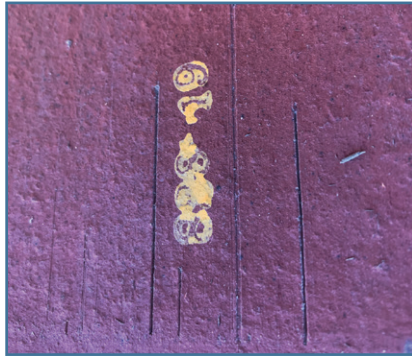
Figure 27: Cosmetic Imperfection (caused by extrusion marks)
