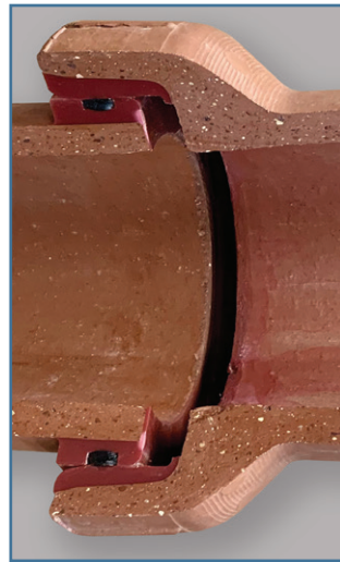
Figure 20: While this joint cutaway shows a significant gap in the pulled joint for illustration purposes, the joint holds and would perform as specified.
