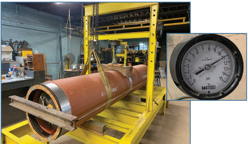
Figure 8: 21-inch VCP Jacking pipe passing the same test.
