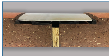
Figure 6: VCP jacking pipe joint.
