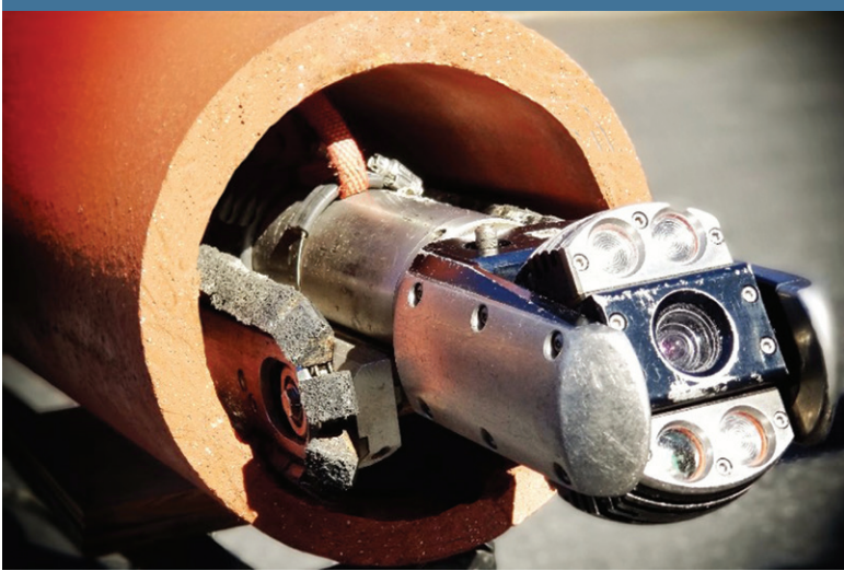
Figure 1: A CCTV camera in an 8" pipe.
