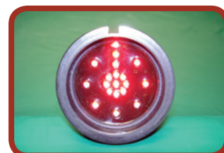
Figure 8-10: LED illuminated target
