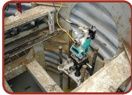
Figure 8-11: Theodolite with camera
