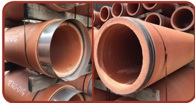
Figure 8-2: Diamond ground pipe end for an elastomeric gasket and stainless steel collar resulting in a low-profile compression joint.
