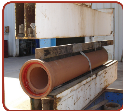
Figure 6-4: In a three-edge bearing test, a 12" pipe is subjected to minimum load of 2,600 pounds per linear foot.
