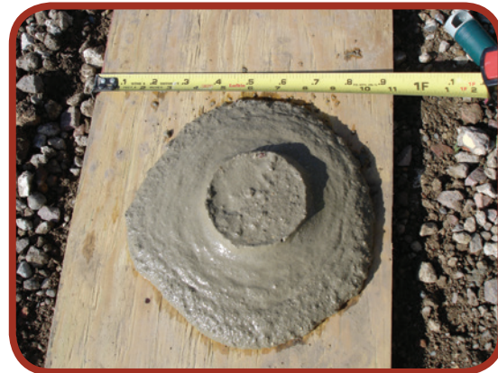
Figure 6-17: Measuring the spread diameter to determine flowability prior to placement.
