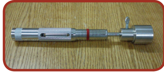
Figure 6-19: A pocket penetrometer can be used to determine CLSM strength prior to backfill
