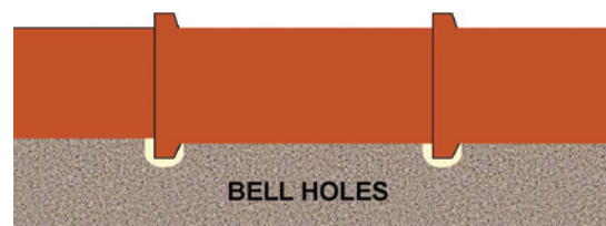
Figure 6-9: Provide uniform and continuous support of pipe barrel between bell or coupling holes for all classes of bedding.
