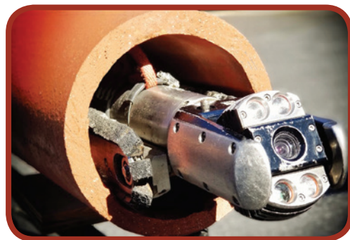
Figure 11-4: A CCTV camera in an 8" pipe. Photo courtesy of Plumbers Depot Inc.
