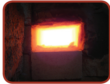
Figure 1-4: Firing at about 2000° F (1100°C) is critical to achieving vitrification which creates a solid pipe body.
