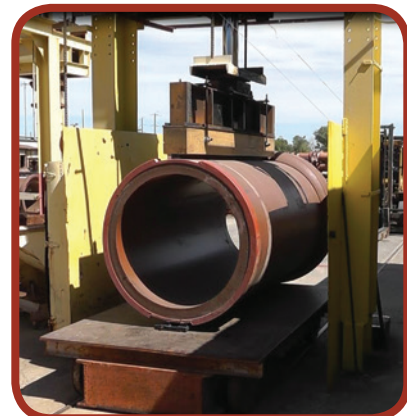
Figure 1-2: Three-edge bearing testing for inherent structural strength.
