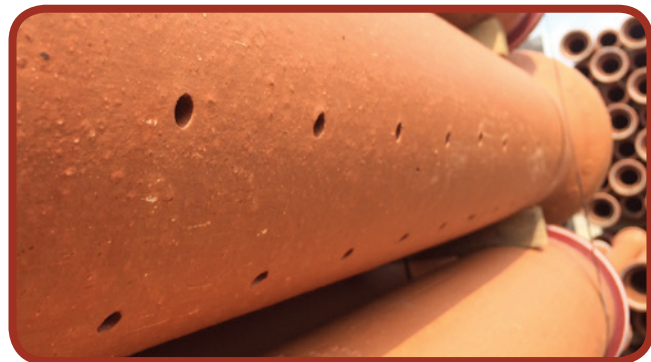
Figure 1-9: Perforated clay pipe is an environmental alternative for drainage applications.
