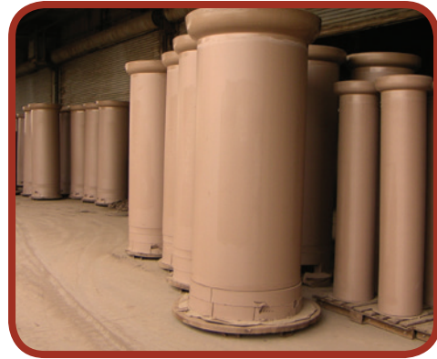
Figure 1-7: Drying rooms capture excess heat from the kilns to help make VCP the most environmentally responsible sanitary sewer pipe product.
