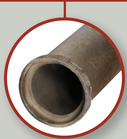
120-year old VCP pipe recently replaced to increase the capacity of the main.
