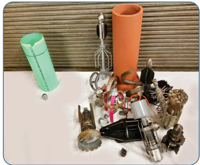
Both PVC and VCP can be cleaned using hydro jets. Only VCP permits the use of mechanical cleaning methods in addition to hydro jetting.
