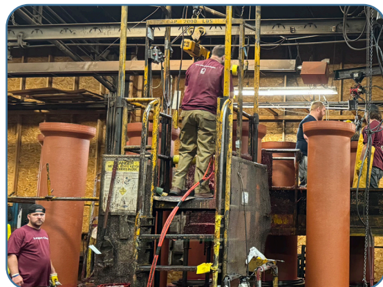
Figure 7: Manufacturing Bell and Spigot VCP Joints
