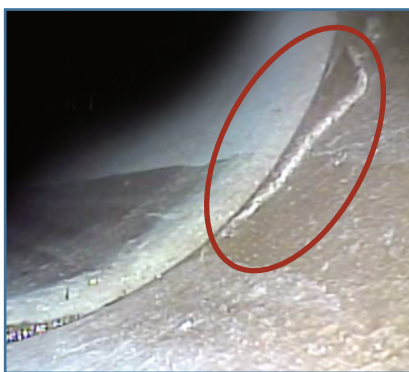
Figure 28: Surface imperfection created during extrusion
