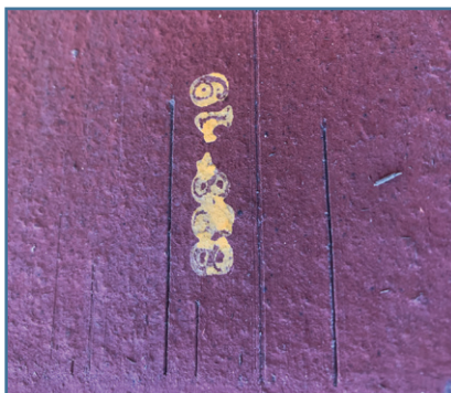
Figure 27: Cosmetic Imperfection (caused by extrusion marks)
