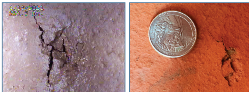
Figure 2: The picture at left was the observed condition of an 8-inch pipe in a CCTV inspection. The photo at right is the recovered pipe that passed the air test. The cosmetic imperfection is well-within the chip allowance specified in ASTM C700 and would have had no impact on long-term performance. For more examples of cosmetic imperfections, see pages 18 & 19.
