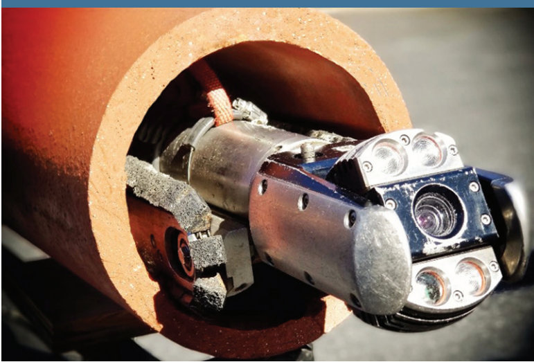
Figure 1: A CCTV camera in an 8" pipe.
